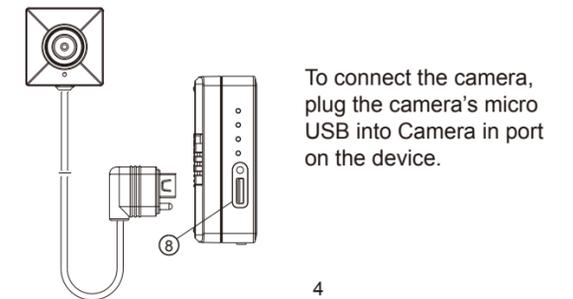
To connect the camera, plug the camera's micro USB into Camera in port on the device.
